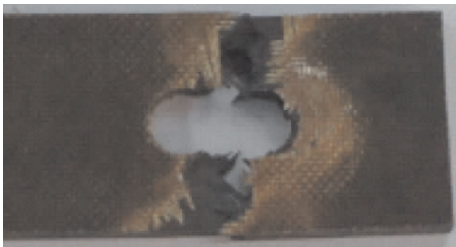
图 8 层合板单钉接头静拉伸试样破坏照片 Fig. 8 Picture of single joint under static tension loading after final collapse
